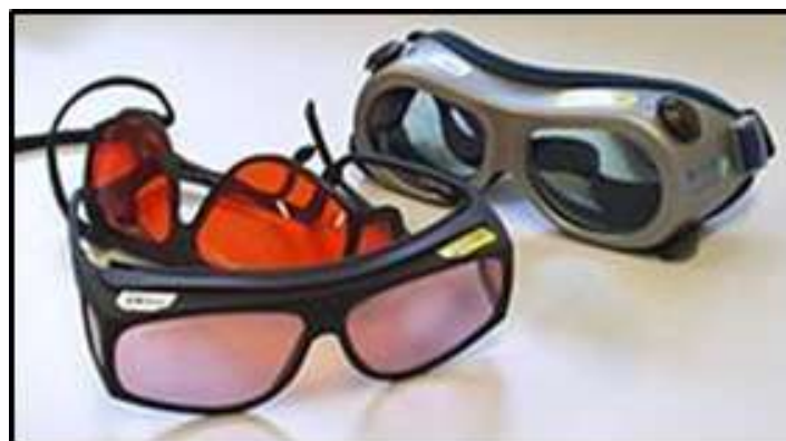
Fig.2. Protective Eyeglasses Used For Different Lasers Depending on the Wavelength of the Laser Beam
